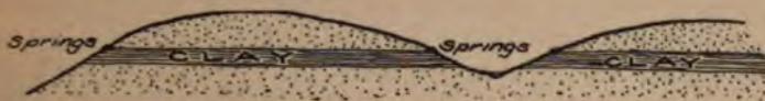
FIG. 189. — Diagram to show how an impervious layer conducts the descending water in a lateral direction to issue in surface springs.
